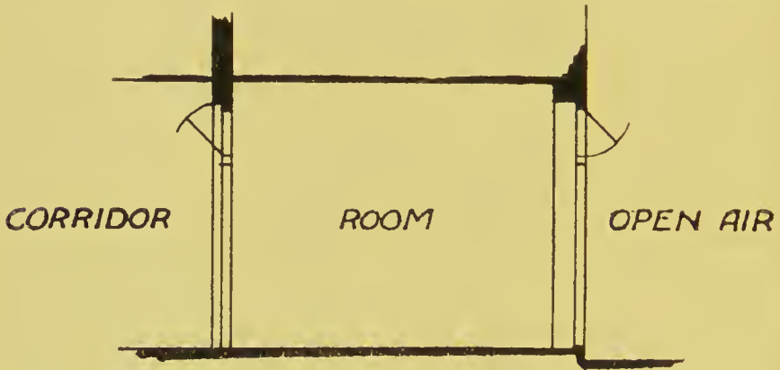
FIG. 18.—VERTICAL SECTION OF SANATORIUM BEDROOM, SHOWING CROSS-VENTILATION THROUGH FANLIGHTS AND OPEN WINDOW.
